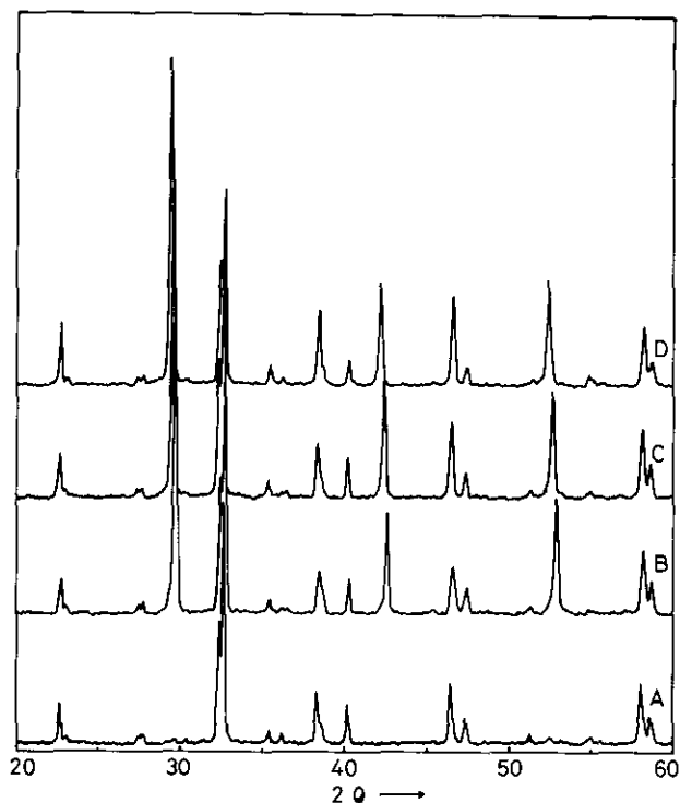
FIG. 5. X-ray diffraction patterns of (A) pure YBCO, (B) 1:1 volume mixture of YBCO and \text{GdBa}_2\text{SbO}_6 , (C) 1:1 volume mixture of YBCO and \text{SmBa}_2\text{SbO}_6 , and (D) 1:1 volume mixture of YBCO and \text{PrBa}_2\text{SbO}_6 , all annealed at 950^\circ\text{C} for 15 hr.
